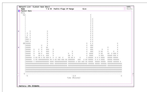
Figure 5.14: The traffic load on one channel over a 5 minute period
