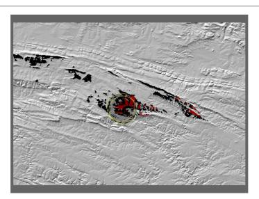
Figure 5.10: An indication of the interference of two APs on each other. The circles indicate the antenna patterns of the two APs while the black area represent an acceptable level of interference and the red very bad signal strength
