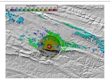
Figure 5.6: The coverage area of an Omnidirectional antenna over Grahamstown. The small round grey area is the location of the AP. While the colored areas depict the coverage
