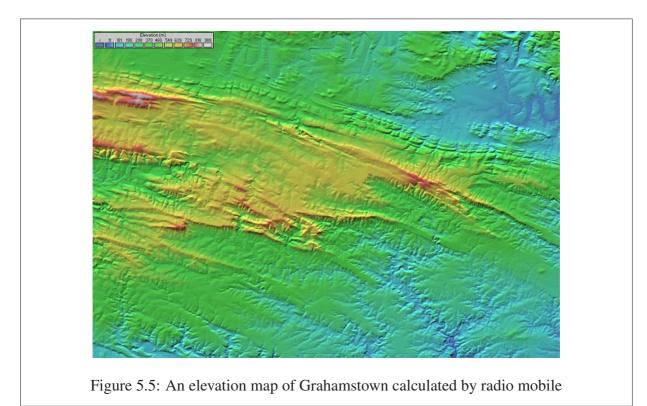
Figure 5.5 is an elevation map of the Grahamstown area with the top left hand corner presenting a color grid of the elevated areas in Grahamstown. Using such elevation data combined with the environment and system parameters, the propagation path can be calculated. Radio Mobile provides the following propagation views:
