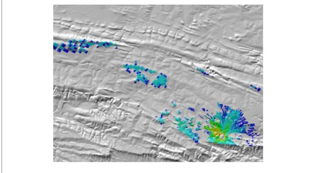
Figure 5.9: A representation of the effect on the signal footprint when the radiation angle of the Yagi antenna are changed to 300 degrees.
